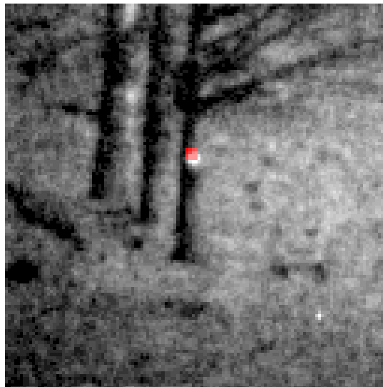
Figure 5: B/W image of the outdoor scene at 128x128 pixel resolution, reconstructed using a subsampling ratio of 18%. The Ø7 cm reflector, seen as a bright dot when the laser is continuously on, is mounted on a tree at 350 m range. The red overlaid image of the simulated 25 ms muzzle flash is reconstructed to 32x32 pixel resolution using 20 consecutive patterns (during a pulse) and illustrates the capability to detect and localize the flash at the same position as the reflector (ground-truth).
